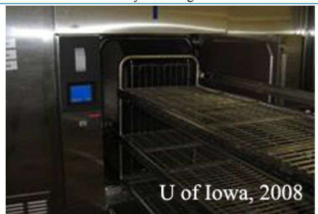
Figure 3B. The final step in the processing of surgical instruments involves steam sterilizing using the autoclave shown below. This is basically a large, modified pressure cooker in which high temperature and high pressure are used to kill any microorganisms.
